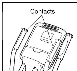
When your pulse is detected, your heart rate will be shown in the display. For the most accurate heart rate reading, hold the contacts for at least 15 seconds.
