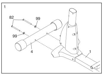
While another person lifts the Folding Frame (2), attach the Rear Stabilizer (3) to the Folding Frame with two M10 x 93mm Button Screws (82) and two M10 Curved Washers (99).
