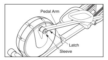
Next, raise the pedal arms until they touch the magnets on the upper body legs; the magnets will hold the pedal arms in place. Then, hold the handle and lift the frame until it locks in a vertical position.
