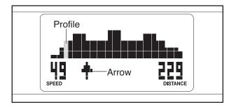
**During both programs,** the console will regularly compare your heart rate to the target heart rate setting for the current segment of the program. If your heart rate is too far below or above the target heart rate setting, the resistance of the pedals will automatically increase or decrease to bring your heart rate closer to the target heart rate setting. Each time the resistance changes, the resistance setting will appear in the display for a few seconds to alert you.
